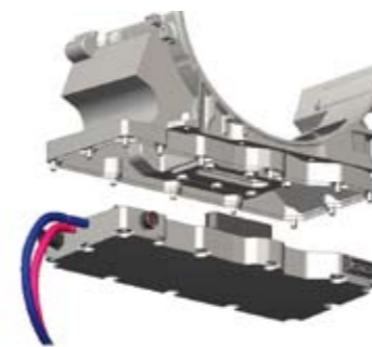
Fig. 5: Partial integration of the power electronic system in the automobile gear unit (EFA-project)
