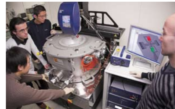
Fig. 3: PVM-200 vacuum wafer prober and microsystem analyzer
