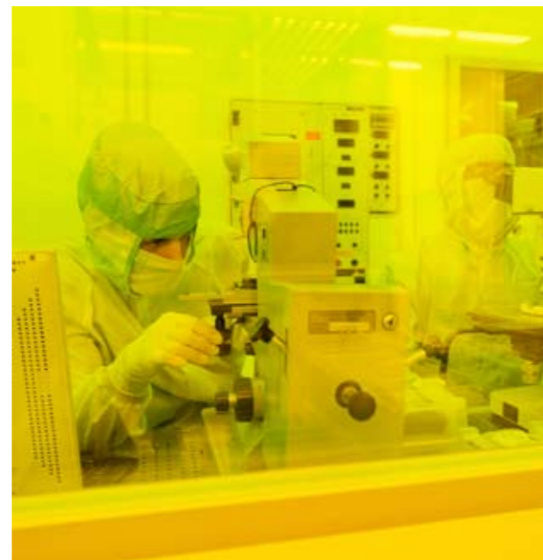
Fig. 1: Wafer inspection within the lithography clean room
