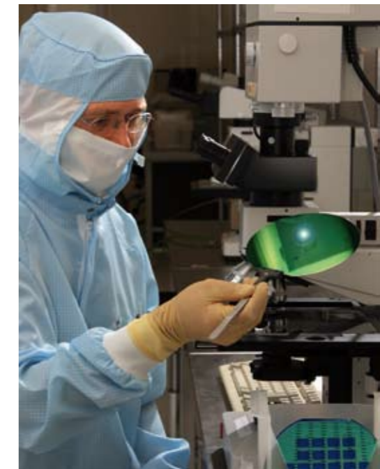
Fig. 3: Wafer inspection at the microscope
